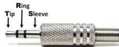
3.5mm 3-Conductor (TRS) Connector
